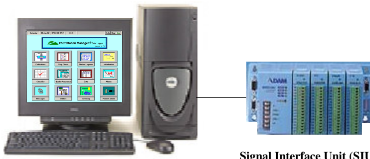
Station Manager Data Logger PC
